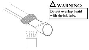
**6** Slide a 76mm (3'') length shrink tube over the braid leaving 12mm(0.5") of shrink tube past the braid. Shrink with heat gun until completely shrunk. While still warm, squeeze the entire width of shrink tube closed.
