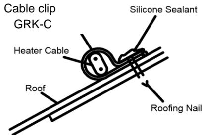
**Asphalt/Shake Shingle Roof** - Fasten with nail, coat nail head and upslope edge of clip with silicone sealant.
