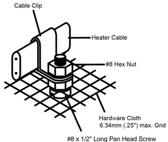
**Flat Roof** - Adhesive (not furnished) should be used to bond clips studs to the flat surface. The roof surface should be clean at the bonding locations. **Do not penetrate flat roofs with screws or nails as leaks may develop.** Allow the adhesive to cure to full bonding strength before attempting to install the cable and clips.
