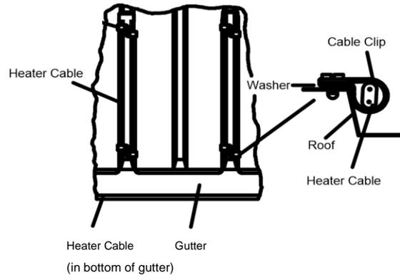
**Metal Roof** - Fasten with sheet metal screw using neoprene sealing washer. If washers are not available, coat screw and upslope edge of clip with silicone sealant. Exact cable spacing may vary depending on the rib design of the roof. Typically trace every other rib.
